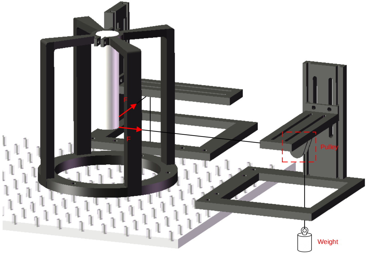
Figure 20: Experimental setup for compliance regulation validation
