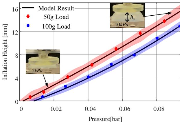
Fig. 8. Results for an inflation of a circular elastic membrane with constant load of 50g and 100g.
