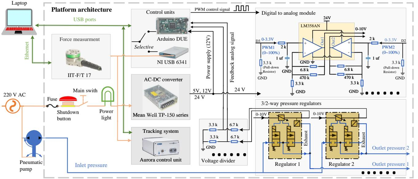
Fig. 5. Connection architecture of the platform. AC power and inlet pressure are provided from external supplies. Data transmission between the laptop and the platform is achieved via USB and Ethernet. Both the Arduino Due and USB-6341 can be selected as the control unit, depending on specific applications.
