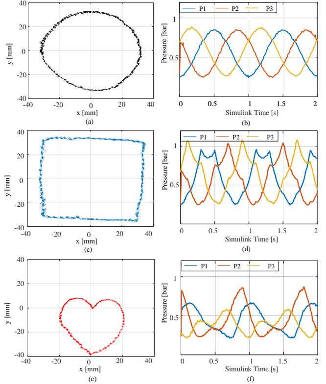
Fig. 10. Results for the inverse kinematics implementation. The Aurora tracking system records the different trajectories of (a) a circular, (c) a rectangular and (e) a heart shape. The recorded control pressure values are plotted in (b), (d) and (f). This Simulink example can be downloaded from the GitHub repository.
