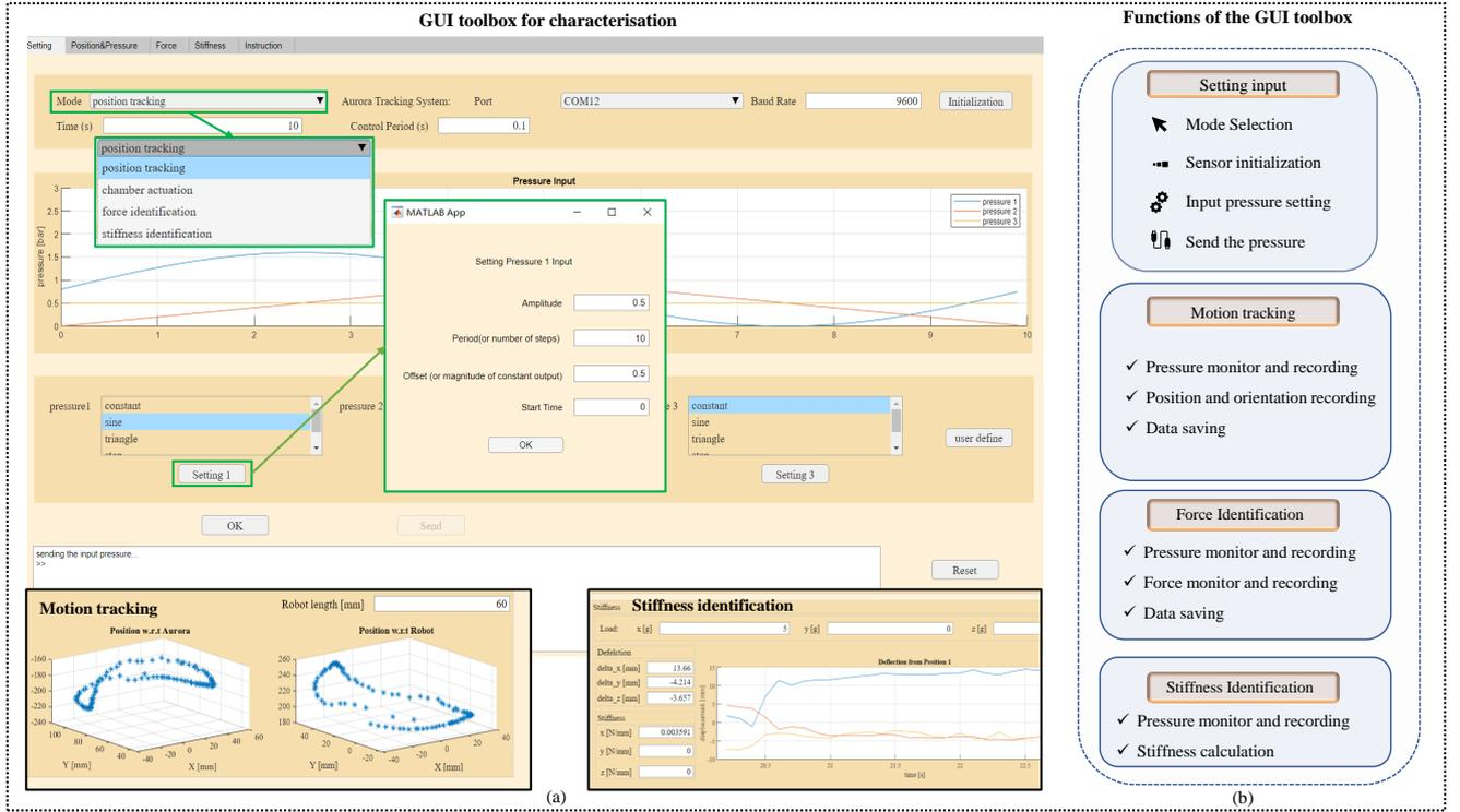
Fig. 6. The design of the GUI toolbox for robot characterisations. (a) Snapshots of the main page for setting, with the motion recording and stiffness identification examples shown at the bottom. (b) The architecture of the GUI. The source codes for the GUI can be downloaded from the GitHub repository.
