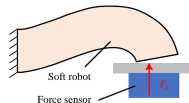
Fig. 3. Example of a blocked force identification setup. The tip of the robot is locally constrained when the robot is actuated. The force  $F_b$  can be measured by a force sensor.
