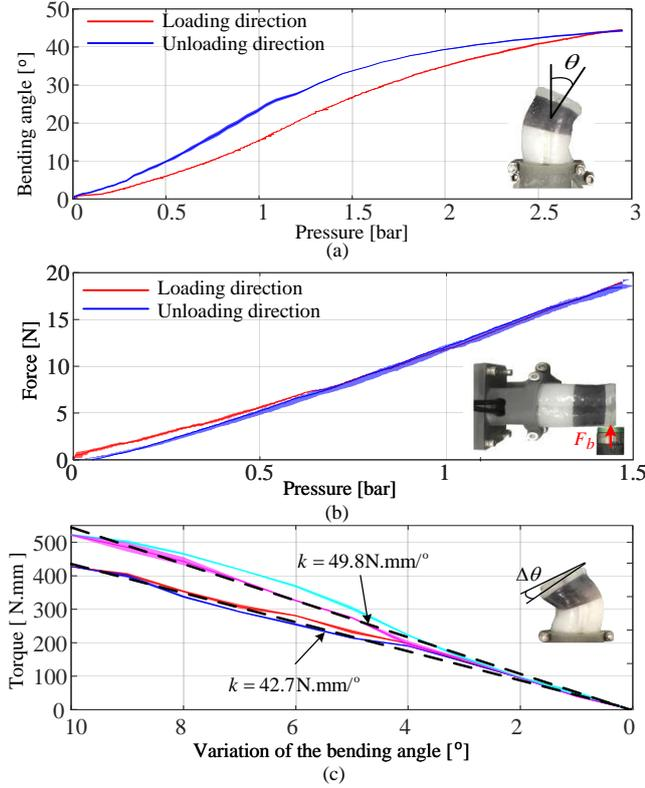
Fig. 7. Characterisation results for the variable stiffness joint. (a) Kinematics identification. (b) Force generation identification. (c) Variable stiffness analysis for two pressure combinations.
