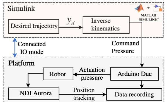
Fig. 9. Control scheme of implementing the inverse kinematics to the platform using Simulink.
