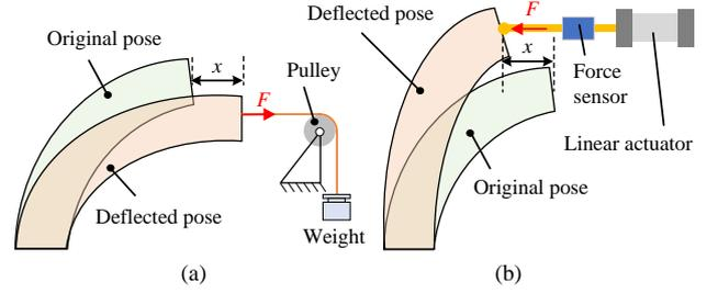
Fig. 2. Stiffness measurement demonstrated on a soft robotic manipulator applying (a) a pulling and (b) a pushing force. The force  $F$  results in a displacement or deflection  $x$  along the force direction.
